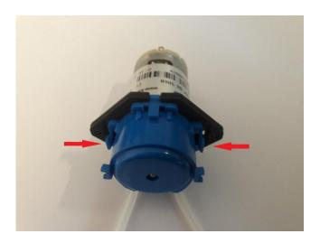
To open the pump module, gently press on the other two clips and remove the pump cover.
