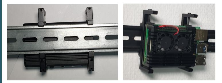
Now you can press the housing clamps onto the top-hat rail and lock them with the screws if necessary.
