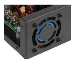
After the cables are connected and the fan is mounted, you can install the small board with two nuts at the case.
