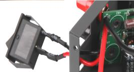
Now you can attach the mainboard with four screws at the bottom of the case and integrate the inputs and outputs of the power supply.
