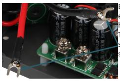
Both sides must be about 5mm at the end stripped because on both ends have to be forked cable lugs attached. These ends should be isolated with shrinking tubes either to prevent shorts.
