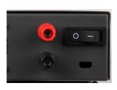
Screw the ports at the case and attach the red ports at the top and the black ones at the bottom like that:
