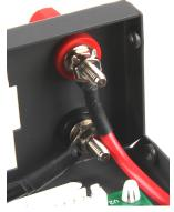
The end of the cable from the output voltage must be conntected with the ports in the front.
