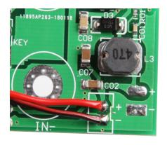
The red cable (+) must be soldered on "+" and the black one (-) on the board at "-".
