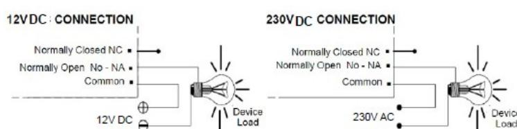
**ABOUT THE OUTPUT.** During operation of the circuit, and according to its load, it could happen a fluctuation or an incorrect operation of the output. If this happens, install an anti-spark circuit between the two contacts of the relay used in the connection.
