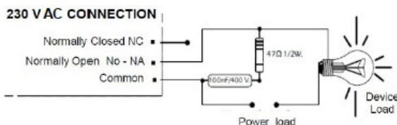
**TIMING AND PERFORMANCE.** Install a push on terminal "Push". In his connection, cable length should not exceed 30 cm. If greater use shielded cable.
