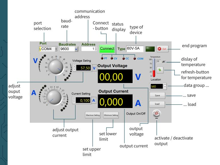
The output is deactivated if the button glows red. It will be green as soon as the output is activated.
