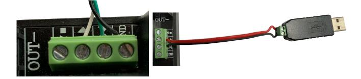
After the cable is connected with the power supply like in the picture and the chart, the device can be connected with the PC via USB. In the device-manager in point "connections (COM & LPT)", the port of the power suppy can be found. In this case, it is COM4.
