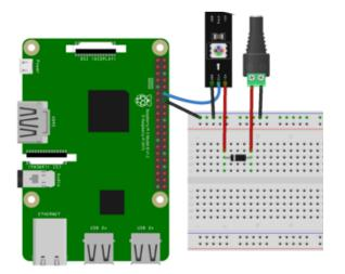
Pi pin 18 to NeoPixel DIN. 1N4001 diode cathode (side with the stripe) to NeoPixel 5V. Power supply ground to Pi ground. Power supply ground to NeoPixel GND. Power supply 5V to 1N4001 diode anode (side without the stripe). Make sure to get the orientation of the diode correct, with the cathode (side with the stripe) going to the NeoPixel!
