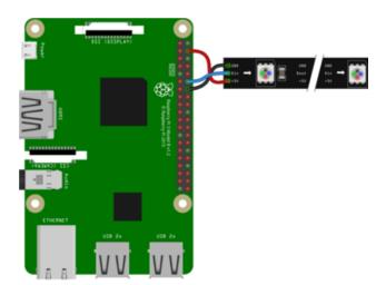
Pi 5V to NeoPixel 5V Pi GND to NeoPixel GND Pi GPIO18 to NeoPixel Din
