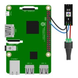
Pi GND to NeoPixel GND Pi GPIO18 to NeoPixel Din Power supply ground to NeoPixel GND Power supply 5V to NeoPixel 5V
