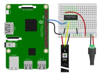
Pi GPIO18 to 74AHCT125 pin 1A 74AHCT125 pin 1Y to NeoPixel DIN Power supply ground to 74AHCT125 ground
