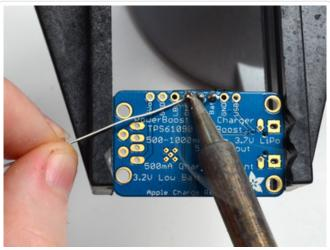
Solder in all three pins with any kind of solder making sure you have a good connection
