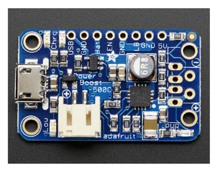
The PowerBoost 500C has at the heart a TPS61090 boost converter from TI (http://adafru.it/duQ). This boost converter chip has some really nice extras such as low battery detection, 2A internal switch, synchronous conversion, excellent efficiency, and 700KHz high-frequency operation. Check out these specs!
