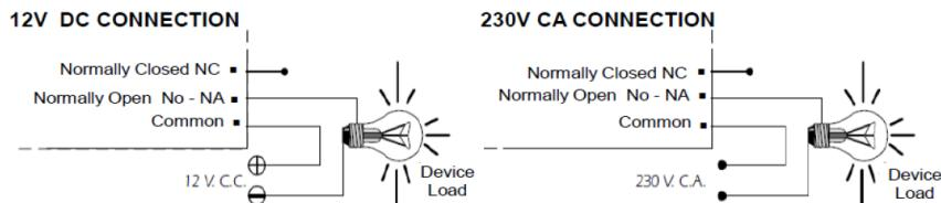
**CONSIDERATIONS ABOUT THE OUTPUT :** During the operation of the circuit, and depending on its load, a fluctuation or an incorrect operation of the output may occur. If this occurs, install a non-sparking circuit between the two relay contacts used in the connection.
