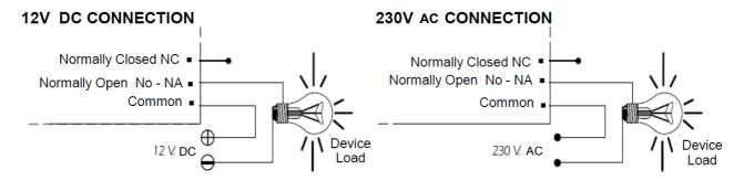
**ABOUT THE OUTPUT.** During operation of the circuit, and according to its load, this could be a fluctuation or an incorrect operation of the output. If this happens, install anti-spark circuit between the two relay contacts used in the connection, as shown in the drawing.
