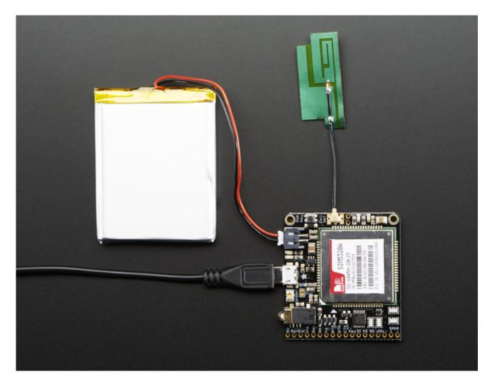
Then press the small **KEY** button next to the battery & cell antenna for 5 seconds. Then the computer will recognize a multi-type USB connection. Install the drivers (http://adafru.it/jFn)
