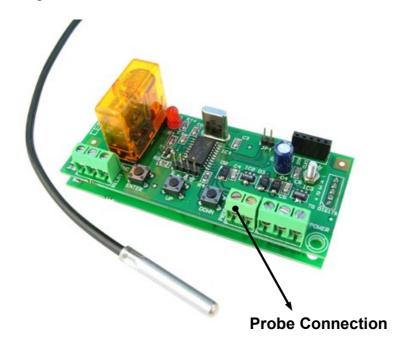
**NOTE.** Connect the 2 wires of the probe connected to the connector labeled probe. Has no polarity probe, you can connect as you want
